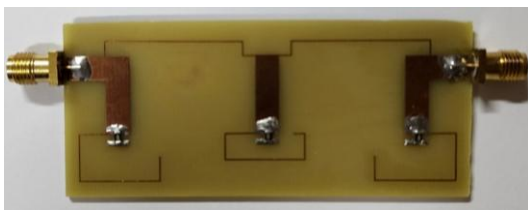
Fig. 13. The three-cell two-port reflectionless BPF. (a) physical dimensions in mm: l_1 = 25.9 , l_2 = 3 , l_3 = 15 , l_4 = 7.3 , l_5 = 5.3 , l_6 = 9 , l_7 = 15 , l_8 = 4.5 , l_9 = 9 , l_{10} = 15 , l_{11} = 6 , l_{12} = 5 , l_{13} = 15 , l_{14} = 5 , l_{15} = 2 , w_1 = 0.3 , w_2 = 4.5 , w_3 = 4.5 , w_4 = 0.3 , (b) photograph.
